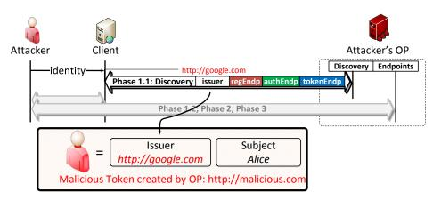
Figure 3.2: Issuer Confusion: The Attacker OP sets the *issuer* parameter to an Honest OP during the Discovery phase. As a result the Client can be confused that the Attacker OP controls the identities of the Honest OP.
