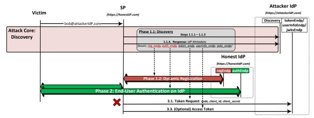
Figure 7: Malicious Endpoints attack: by manipulating the Discovery, the attacker steals the code.
