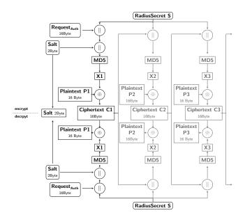
Fig. 3. RADIUS encryption and decryption
